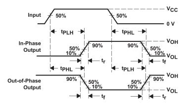
Figure 3. Propagation Delay and Output Transition Times
